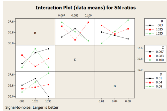
Fig. 5 Interaction Plot for S/N ratios of Surface hardness
